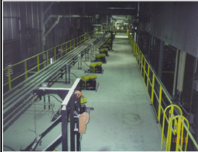
Left - An annealing lehr showing several of our fans in service
