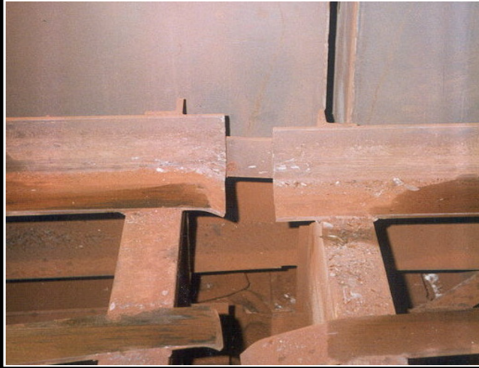
Right - Two frames inside of a tunnel furnace that are misaligned.
